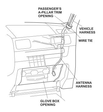
20. Inside the glove box opening, route the antenna harness along the vehicle harness towards the driver's side of the vehicle. Secure the antenna harness to the vehicle harness with three wire ties in the areas shown.
