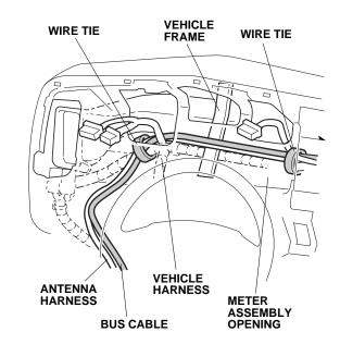
37. Align the end of the bus cable connector with the end of the vehicle 20-pin connector and secure the bus cable to the vehicle harness using a wire tie.
