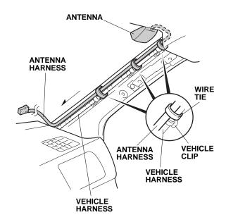
17. Using a felt-tip pen, mark the antenna harness at the point where the harness touches the dashboard.
