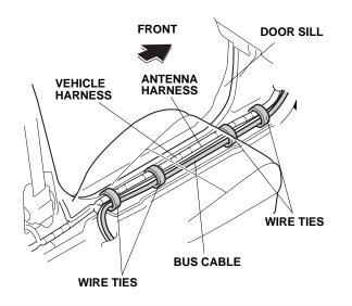
35. Route the bus cable along the antenna harness as shown. Secure it to the vehicle harness by tightening the four wire ties loosely-installed in step 24.
