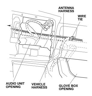
22. Route the antenna harness as shown and secure it to the vehicle harness with two loosely-installed wire ties.
